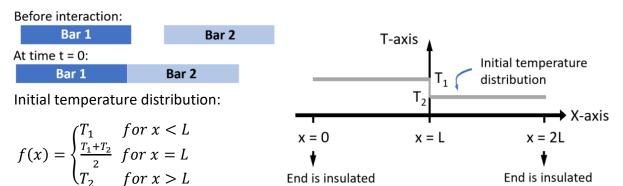
The problem satisfies the below heat conduction equation and with u(x, t) the temperature at any time and place in the joined metal bars as in Eq. (1). Further, because the bar ends not in contact are isolated, the following condition in Eq. (2) holds:
