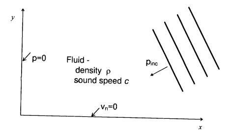
A continuous sinusoidal plane wave  $p_{inc}(\mathbf{r},t) = p_0 \cos(k_x x + k_y y - \omega x)$  is incident at an arbitrary angle on two orthogonal semi-infinite planes as shown above (note that  $k_x$  and  $k_y$  are negative real numbers.) The x-z plane is rigid and immovable  $(v_n=0)$  and the y-z plane is pressure release (p=0).
