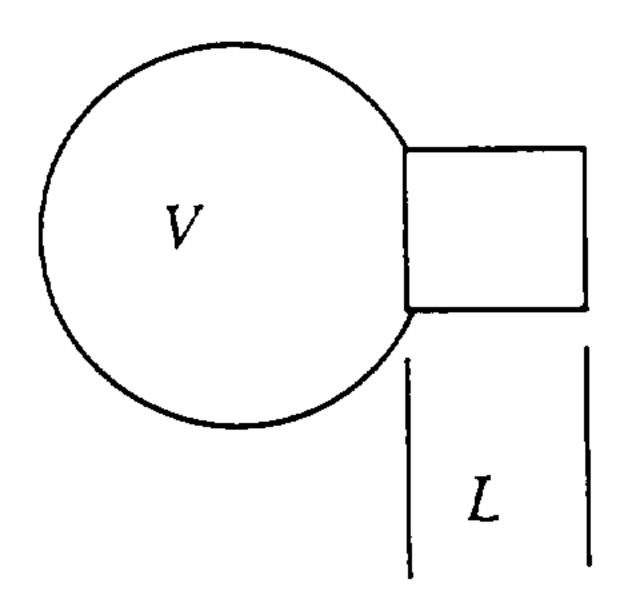
1. A Helmholtz resonator is classical lumped-element acoustic device (anytime you've blown air across the end of a bottle and generated a tone, the bottle is acting as a Helmholtz resonator). Consider the resonator at left. It is a hollow sphere with volume V and a neck of length L. The neck has a cross section area A, and is open (i.e., air can flow into and out of the sphere through the neck).
