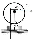
A bicycle is traversing a circular path of radius R at a constant speed **v** and lean angle of  $\theta$ . The front wheel of the bicycle shown in the figure has radius *r*, polar moment of inertia  $I_{zz}=J$ , and axial moment of inertia  $I_{xx}=I_{yy}=I$ . Assuming the wheel rolls without slipping, find
