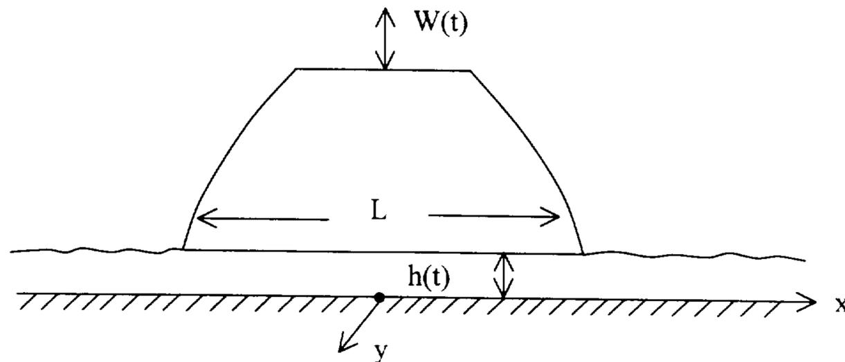
Consider a two-dimensional thrust bearing (very long in the  $y$ -direction) that is supported by an oil film of thickness  $h$ , as shown above. The load on the bearing oscillates such that the film thickness is given by
