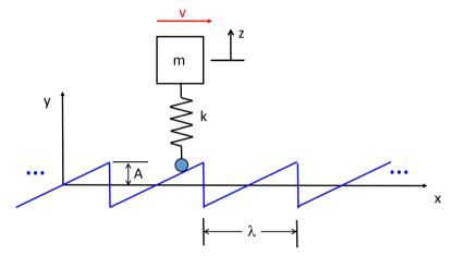
(c) Give a sketch of the "amplitude" of z(t) vs the speed v of the vehicle. Identify the locations of any peaks. You may assume that the speed is varied very slowly.
