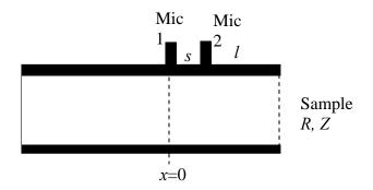
1) Considering plane waves of frequency  $\omega$  incident from the left, derive an expression for the complex reflection coefficient of the sample in terms of the transfer function between the two microphones,
