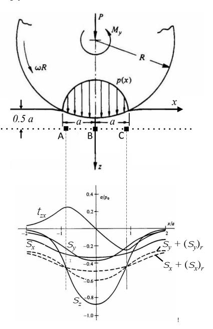
$(S_y)_r$ , respectively, are generated. These altered stress components are shown as the dashed curves in the stress plot. How has the maximum shear stress at location B changed from the initial condition? Is it higher, lower, or unchanged? Justify your answer.
