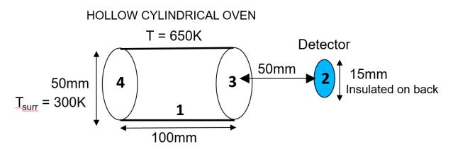
Consider the cylindrical oven (surface 1) shown above which is black and at a constant temperature of 650K, open at both ends (surfaces 3 and 4) to surroundings at 300K. A detector of circular shape (surface 2) is placed a distance of 5cm away from the oven on the center axis of the cylinder. The detector is opaque diffuse and gray with emissivity 0.5.
