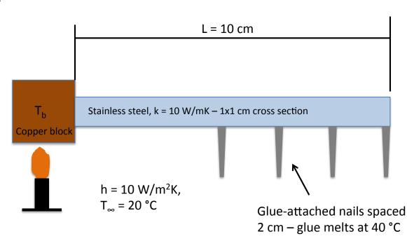
You designed an experiment with simple supplies to convey important heat transfer concepts to high school students. A long, square cross section steal rod is welded to a copper block that is heated with a flame to a constant temperature,  $T_b = 100$  °C. Four nails are glued (melting temp of glue is 40 °C) to the rod spaced by 2 cm from the end of the rod. The ambient conditions are fixed as given – radiation can be neglected.
