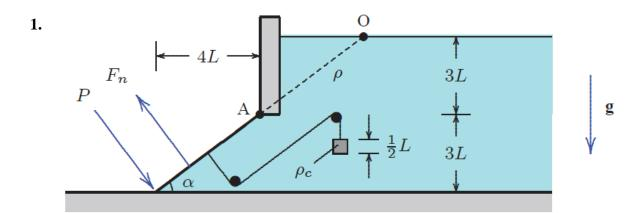
A rectangular gate of width 6L out of the page is hinged at point A and holds back a fluid of density  $\rho$  as shown. A cube of density  $\rho_c = 5\rho$  and side  $\frac{1}{2}L$  is connected to the gate through its centroid with a pulley arrangement so that the weight exerts a force normal to the gate. Neglecting the weight of the gate, determine the minimum force, P, required to hold the gate closed in terms of  $\rho$ , L and gravitational acceleration, g.
