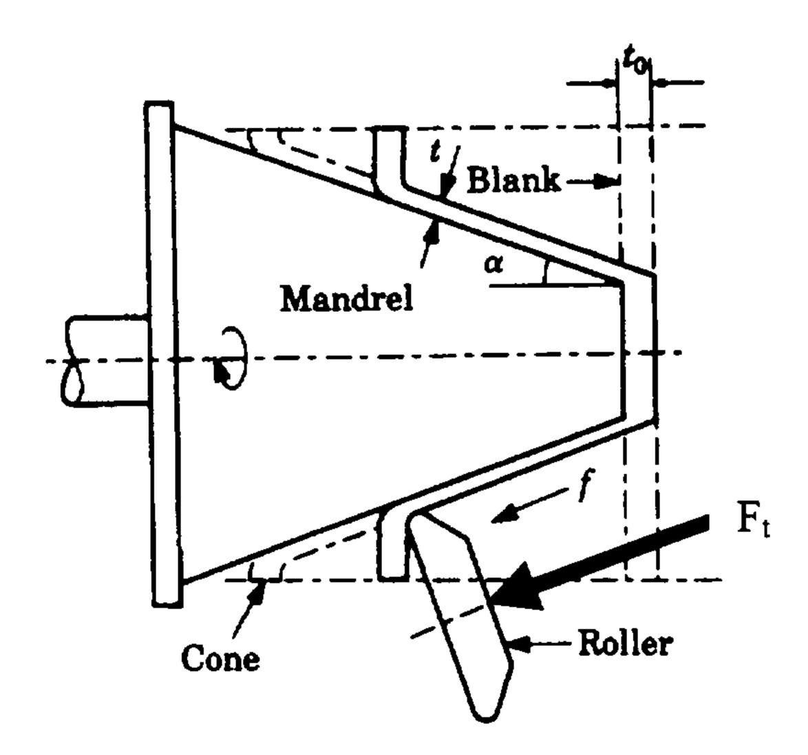
In shear spinning over a conical mandrel, the thickness of the spun part is given by
