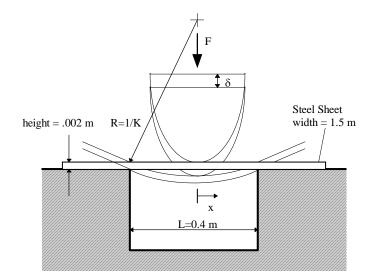
(a) Determine the maximum curvature, K achieved for a punch load of F = 3000 N.
