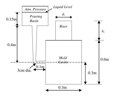
(a) Estimate the time it will take to fill the 0.3m diameter cylindrical mold cavity. Neglect the time required to fill the runner and riser and assume that throughout mold filling the height of molten metal in the pouring basin is kept constant. Clearly state all assumptions you make in arriving at the answer. <u>Note</u>: the dashed line in the above figure serves to indicate the location of the gate relative to the entire mold cavity.
