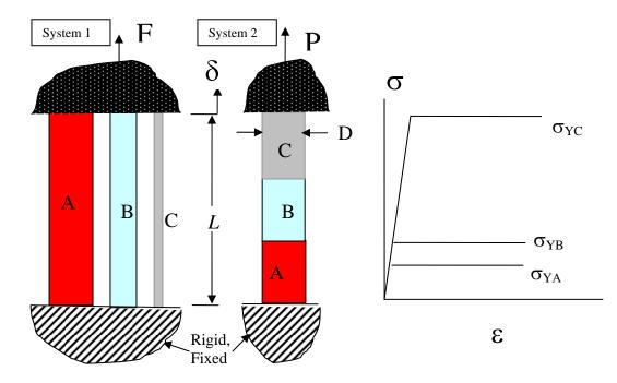
In the diagram shown above, three materials (A, B, C) exhibit elastic-perfectly plastic behavior shown above (right) with yield strengths  $\sigma_{YC} = 450 MPa$ ,  $\sigma_{YB} = 150 MPa$ ,  $\sigma_{YA} = 90 MPa$  and Young's moduli of  $E_C = 200 \text{ GPa}$ ,  $E_B = E_A = 70 \text{ GPa}$ . Systems 1 and 2 represent different structural arrangements of these materials to carry the load between plates.
