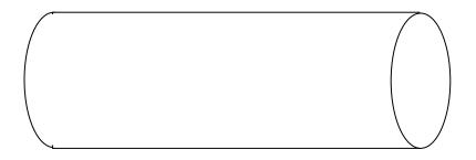
a. Utilize geometry to develop an expression for the strain in the rod as a function of the radius, length, and angle of twist. Give an expression for the maximum strain and show where it occurs. (You must label the changes in geometry associated with twisting the rod on the above sketch. Clearly show the geometry change along the length and along the radius.)
