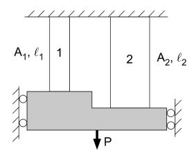
(a) Please derive the relationship between the axial stress,  $\sigma_1$ , and strain,  $\varepsilon_1$ , in Bar 1 in terms of the force, P, the dimensions of the bars, and the elastic modulus of Bar 2. For this part, assume the stresses in the bars are zero when P = 0 and that the temperature is constant.
