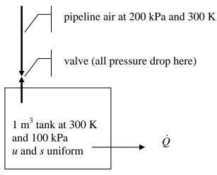
Assume the air in the tank is kept isothermal by heat transfer and that the flow rate of air into the tank is 0.1 kg/sec. Note or recall that the first Gibbs equation may be written as
