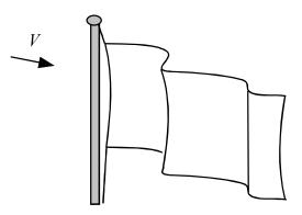
Wind blowing past a flag causes it to "flap" in the breeze. The flapping frequency  $\omega$  is assumed to be a function of the wind speed V, air density  $\rho$ , gravitational acceleration g, length of the flag L, and the "area density"  $\rho_A$  (which has dimensions  $M/L^2$ ) of the flag material.
