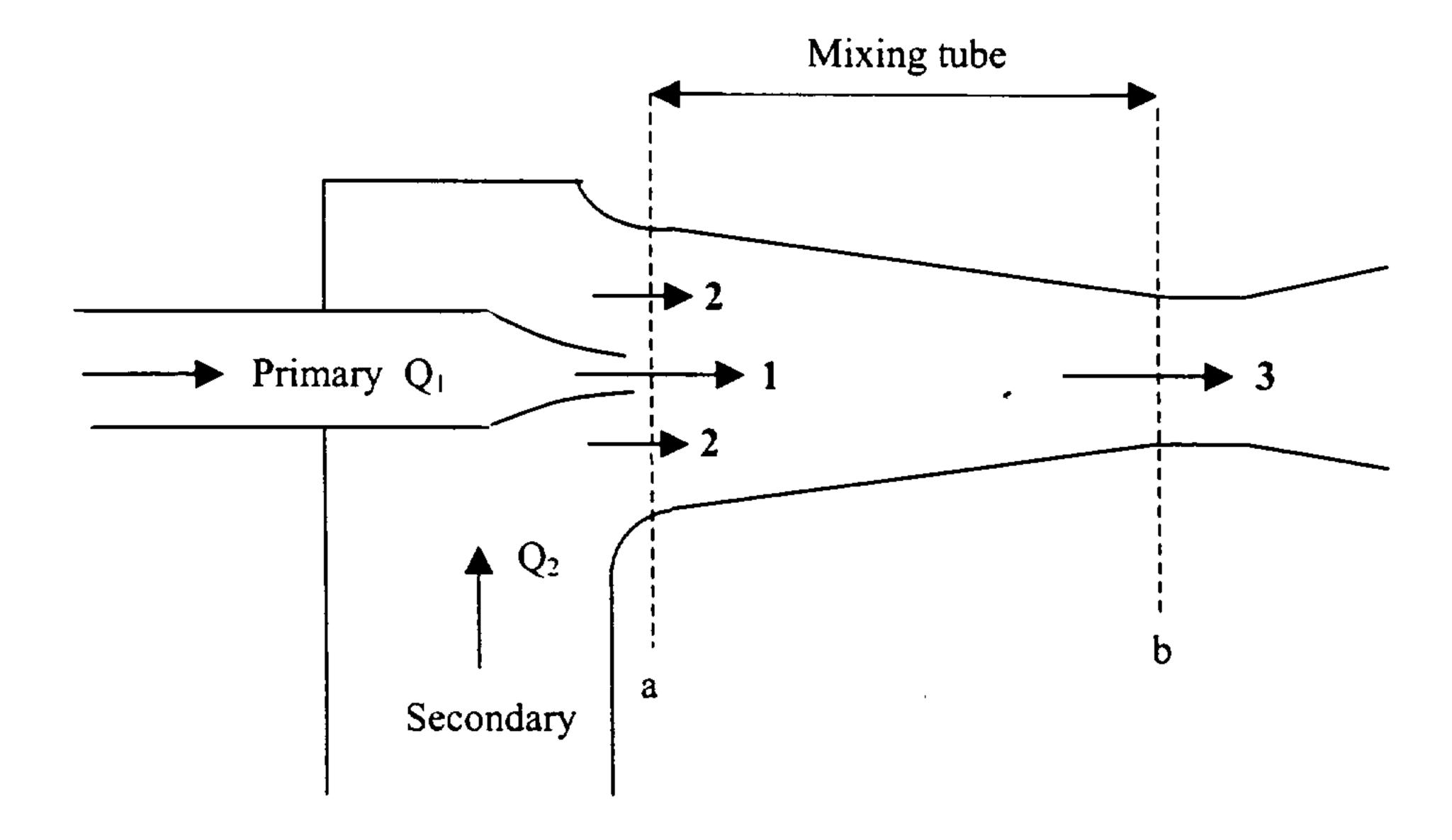
The sketch shows the horizontal mixing tube of a jet pump in which a primary high-velocity water stream entering the mixing tube at section 1 entrains a secondary low-velocity water stream entering at section 2.
