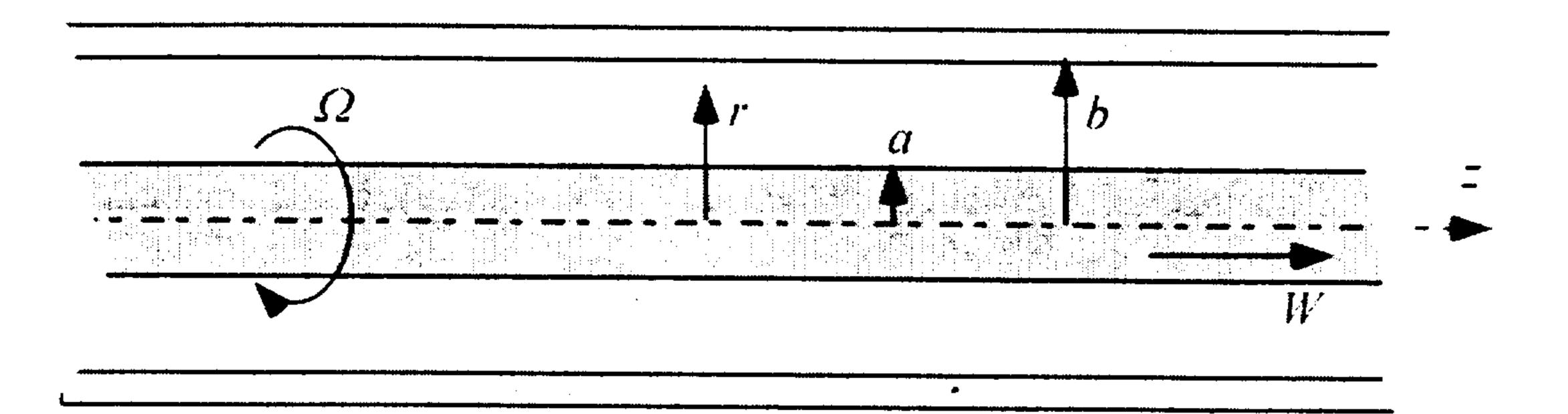
An infinitely long annulus  $a \le r \le b$  is filled with a viscous fluid of density  $\rho$  and viscosity  $\mu$ . The outer cylinder is fixed but the inner cylinder rotates with angular speed  $\Omega$  while translating along its own axis with speed W. The Navier-Stokes and continuity equations are, in cylindrical coordinates,
