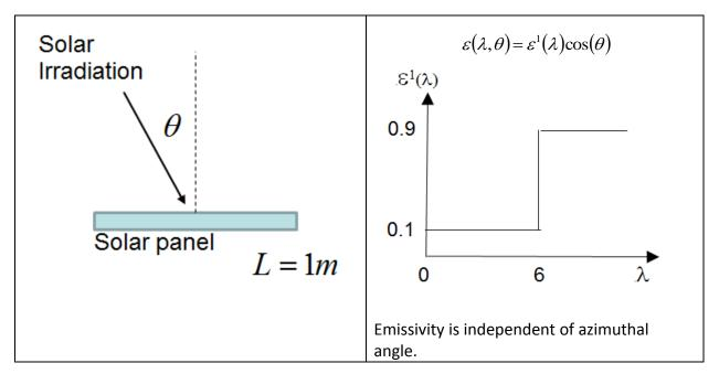
A solar electric panel is mounted on the roof and has incident radiation from the sun at an angle of 30 degrees. The panel has directional spectral emissivity properties given above. Solar irradiation is 1388 W/m<sup>2</sup> and sky temperature 300K.
